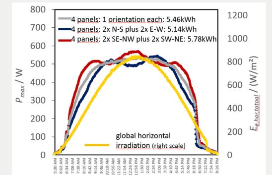
**Fig. 4: Numerical simulation of superposition of different orientations**
