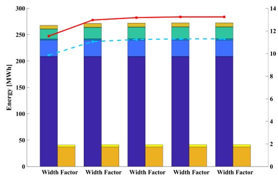
**Figure 2:** Impact of the view fields' width (corresponding to the building land's width) on the annual energy yield.
