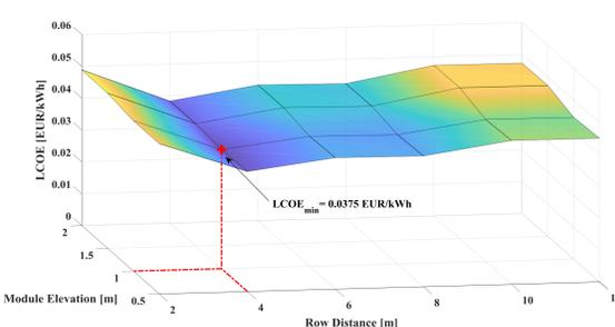
**Figure 4:** LCOE. The red cross indicates the PV field's configuration yielding minimal LCOE.
