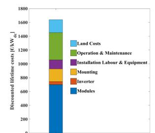
**Figure 7:** Cost breakdown of PV power plant's configuration achieving LCOE<sub>min</sub>
