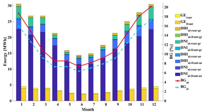
**Figure 1:** Simulated absorbed irradiation, generated electricity, BG<sub>ai</sub> and BG<sub>el</sub>
