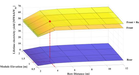
**Figure 6:** Specific electricity yield (regarding front-side capacity) over lifetime.
