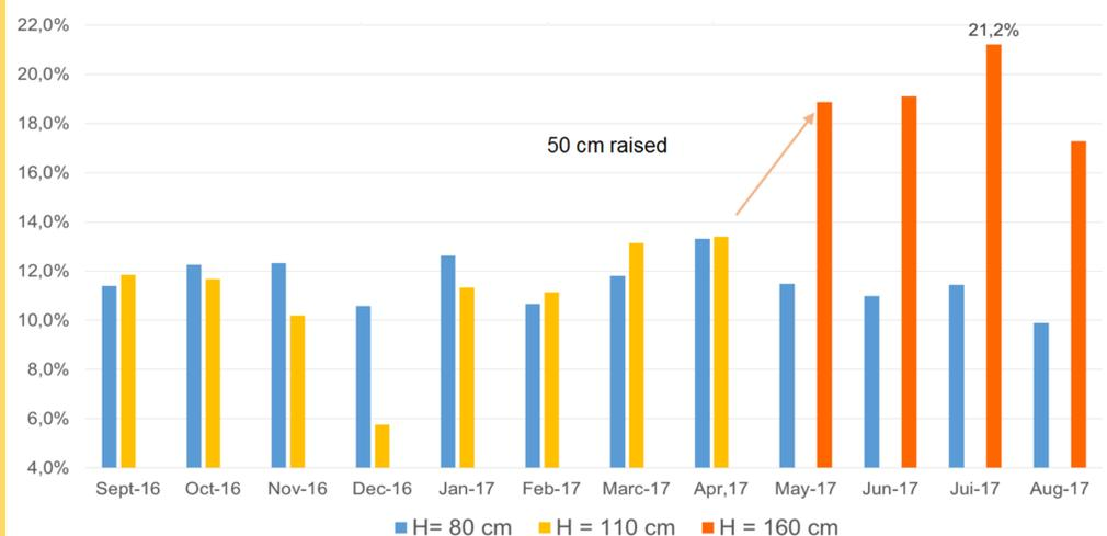
Figure 5: Bifacial Gain for different heights (system 4) vs reference system "R"
