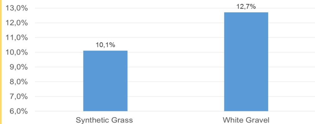
Figure 4: Bifacial Gain on the left grass (albedo ≈ 0,2 – system 1) and on the right white gravel (albedo ≈ 0,4 – system 2) vs reference system "R"
