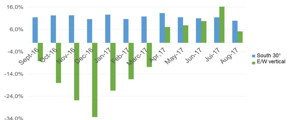
Figure 6: Bifacial Gain for the average of 30° tilted system and E/W vertical system vs reference system "R"
